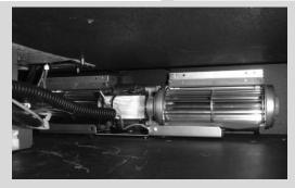
4. Align blower assembly with vibration-damping grommets (shown in step 12) on the base of the appliance. Push the blower assembly backwards to seat the assembly into grommets.
