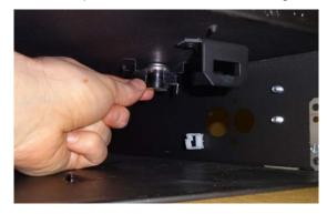
3. Attach the rheostat box mounting bracket to the side of the unit using two of the included screws. The bottom hole on the bracket will fit over the pop rivet on the unit.
