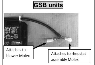
The Molex on the Electrical Controls Assembly attaches to the Molex on the rheostat assembly. There is an additional Molex that comes off of the Electrical Controls Assembly that will attach the Molex on the blower wire harness.
