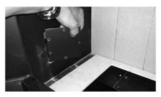
5 Detach the power supply electrical box from the fireplace base by pulling it straight up (it is secured to the base with Velcro).
