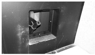
12. Unpack the igniter assembly, place the white square gasket onto the igniter mounting box then connect the air tube to the brass nipple on the igniter.
