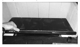
3. Remove the heat shield bolts (2 - 7/16" bolts) and remove the heat shield by sliding to the left and lifting out.
