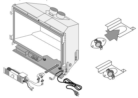
5. Attach the grounding wire from the blower assembly to the power cord mounting bracket. Attach the molex connector from the blower assembly to the power cord as shown below.
