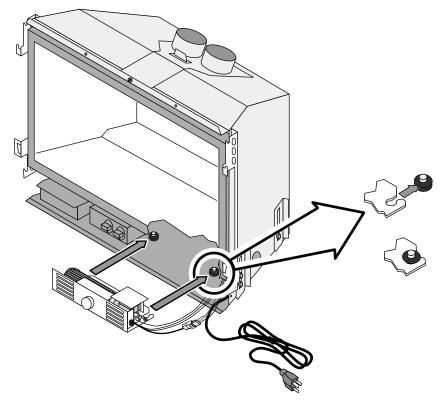
7. Plug the blower in and verify operation. The blower will turn on after the insert reaches temperature, typically 5 to 10 minutes after startup on high.
