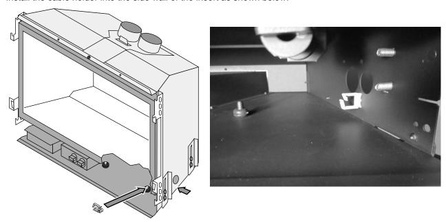
3. Attach the power cord bracket to the insert with the included screw as shown below. Make sure to use the hole to the rear (the front hole is used for the listing tag chain).
